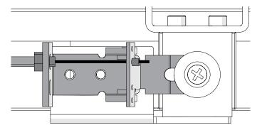
Fasten the manual unlocking lever in the desired position using the hole  ${\bf F}$ .
