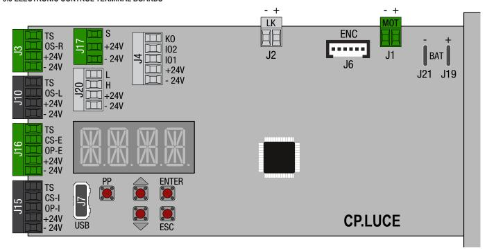
When you connect the safety devices, remove the jumpers of the corresponding terminals.
