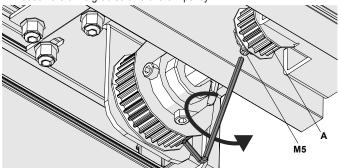
2 - Loosen the 4 M6 screws and move the return "B" in the direction of the arrow until it is disconnected from the A pulley.
