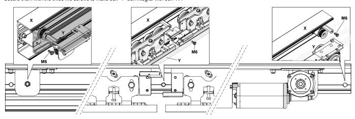
Install the fast leaves "V", bring the leaves to the closed position and make adjustments in height and depth by adjusting their position and overlaps "S" with respect to the slow leaves "L".
