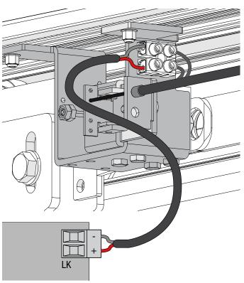
**5.4** - Connect the electric lock output to the LK terminals of the command control unit.
