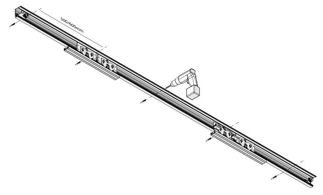
Check/adjust the anti-derailment wheel (a) as shown in the figure. Loosen the screws (C), adjust the vertical position of the leaf using the screw (b) block with the screws (c).
