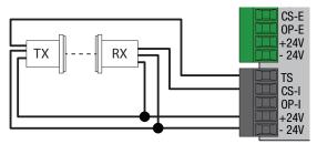
If the TS is not connected, set menu parameter ADV > TS = NO For further information, refer to the installation manual of the photocell.
