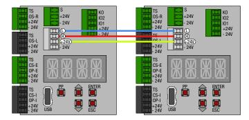
Example of wiring 4 automations (case of two synchronized and interlocked automation groups):
