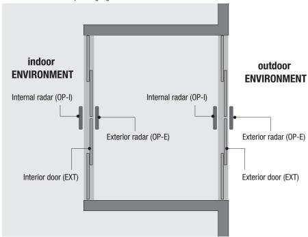
Starting from the rest state, in which both automations are closed, the first to receive an open command starts the opening manoeuvre. The other automation, on the other hand, goes into the 'locked' state where it does not accept any opening commands from the OP-I OP-E contacts. It is however possible to open (for safety reasons etc) using the KO priority open command.
