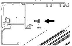
Secure them with the three M6 screws to make box "Y" box integral with box "X".
