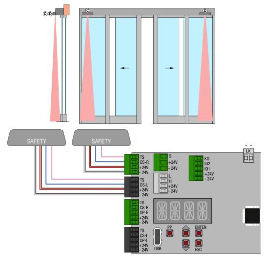
Connect the sensor, using the cable supplied, to the terminals of the electronic control as follows:
