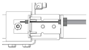
Fasten the manual unlocking lever in the desired position using the hole  ${\bf F}$ .
