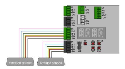
Connect the sensor, using the cable supplied, to the terminals of the electronic control as follows:
