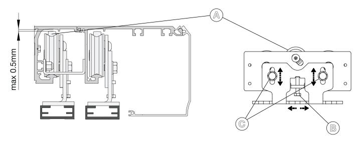
Move the doors by hand for the entire stroke, check that the movement is free and without friction and that all the castors rest on the sliding profile.
