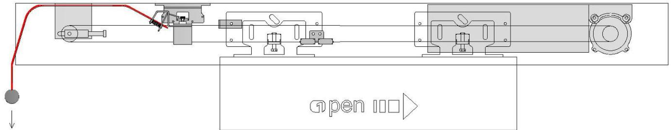
The LUCE R automation is used in emergency exits, and allows automatic opening of the door in the event of a fault, in a power failure, or signalling by an alarm system.
