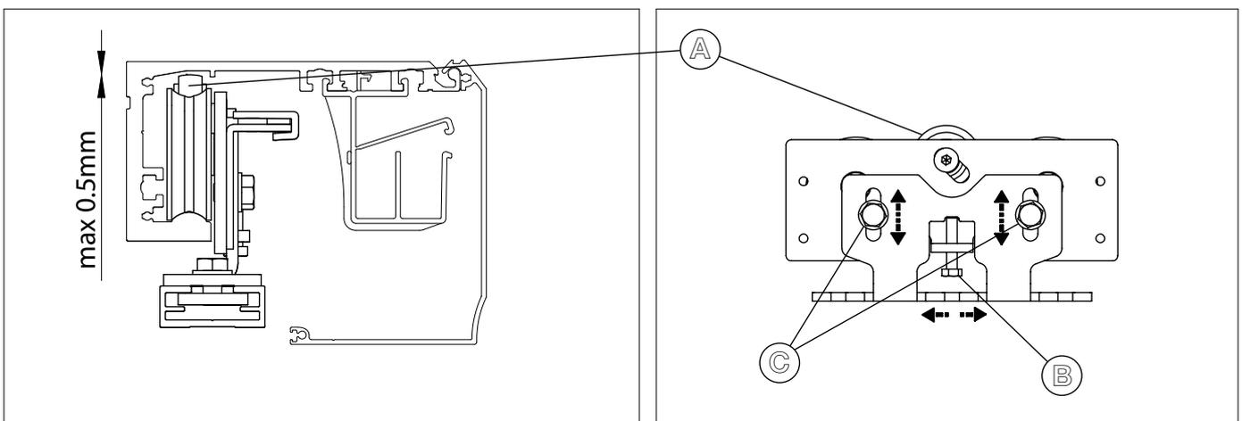
Move the doors by hand for the entire stroke and check movement is free and without friction and that all the castors rest on the sliding profile.
