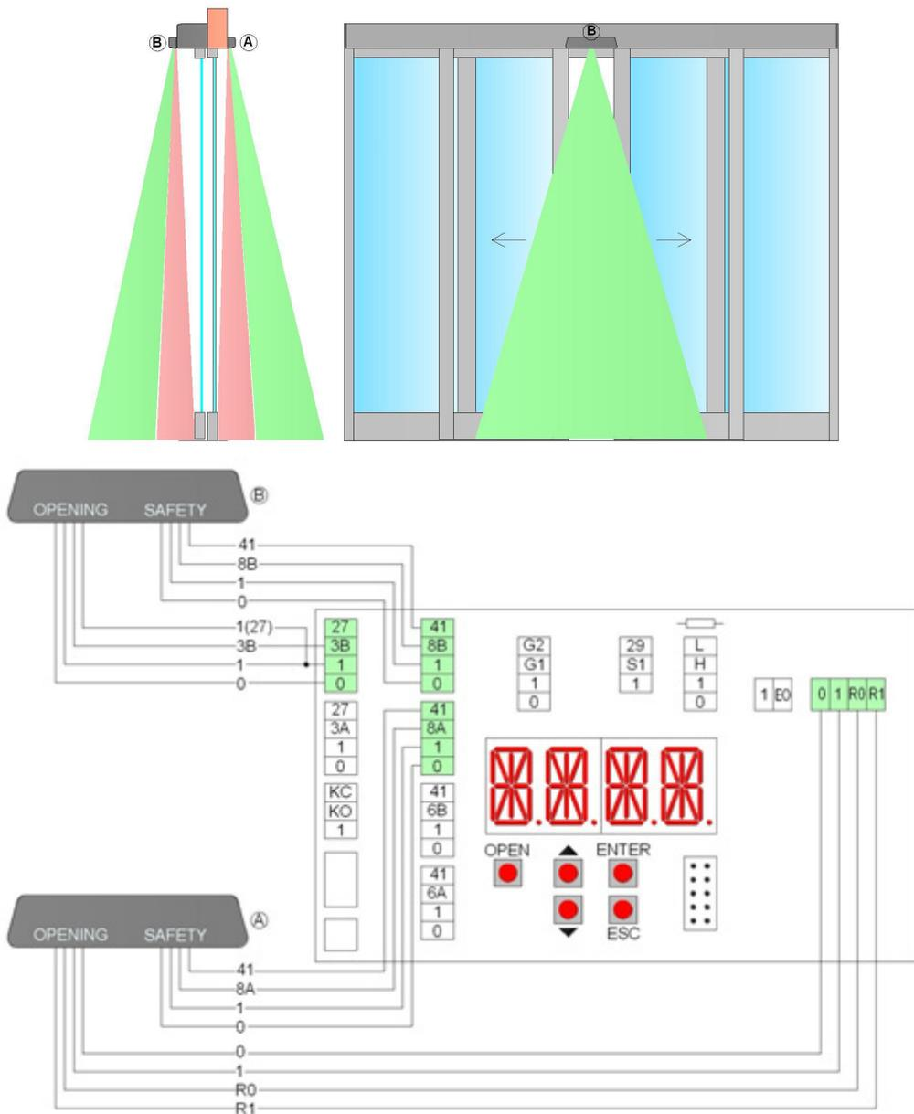
Connect the sensor, using the cable supplied, to the terminals of the electronic control as follows:
