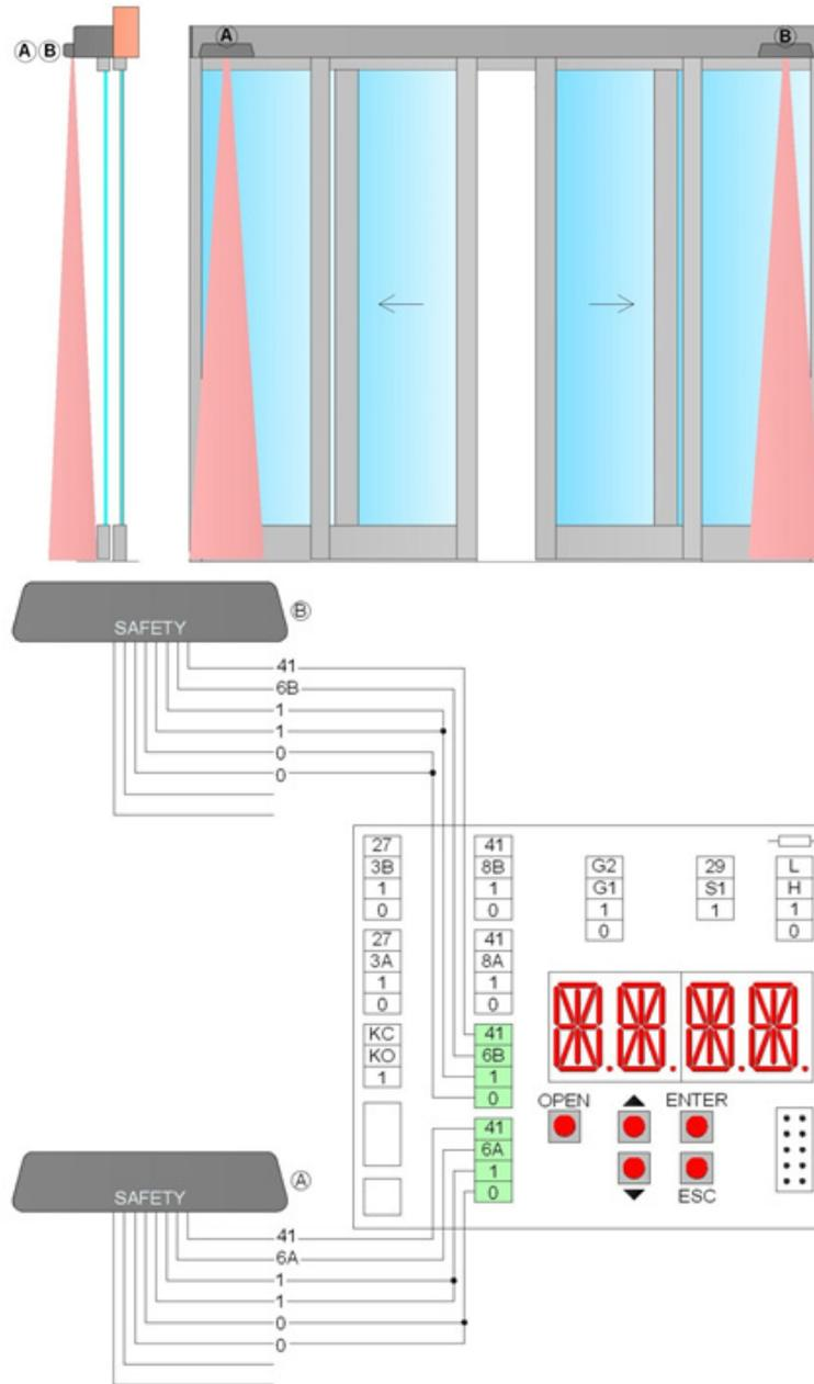
Connect the sensor, using the cable supplied, to the terminals of the electronic control as follows:
